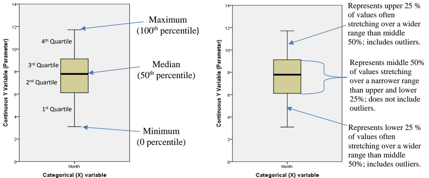
**Figure 2:** General overview of interpreting box plot graphs. Note: The Y axis represents the concentration of a specific parameter and is usually a continuous variable (can take on any positive value). The X axis represents the month when the measurement was taken. It is a categorical variable because measurements can be classified as being taken in one of three months (May, August, and October). Information adapted from (Gotelli & Ellison, 2004).
