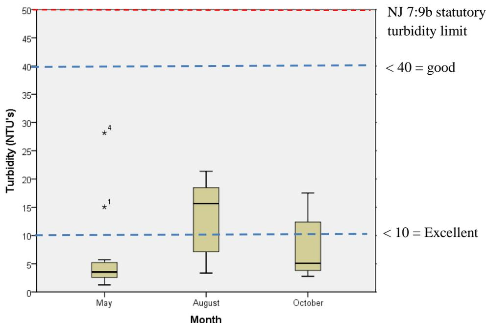
**Figure 8:** Box plots of average turbidity of the lake water for all locations at one foot water depth. Data collected from 2004 – 2016.
