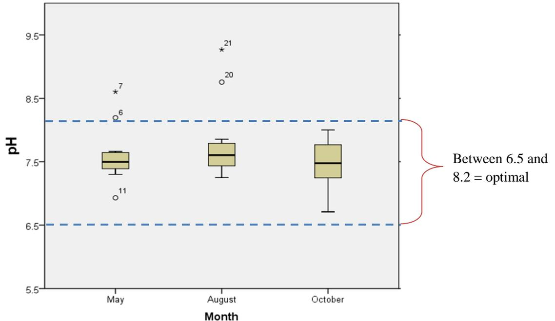
**Figure 7:** Box plots of average pH (acidity) measurements for all locations at one foot water depth. Data collected from 2004 – 2016.
