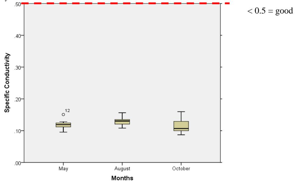
**Figure 6:** Box plots of average specific conductivity measurements for all locations at one foot water depth. Data collected from 2004 – 2016.
