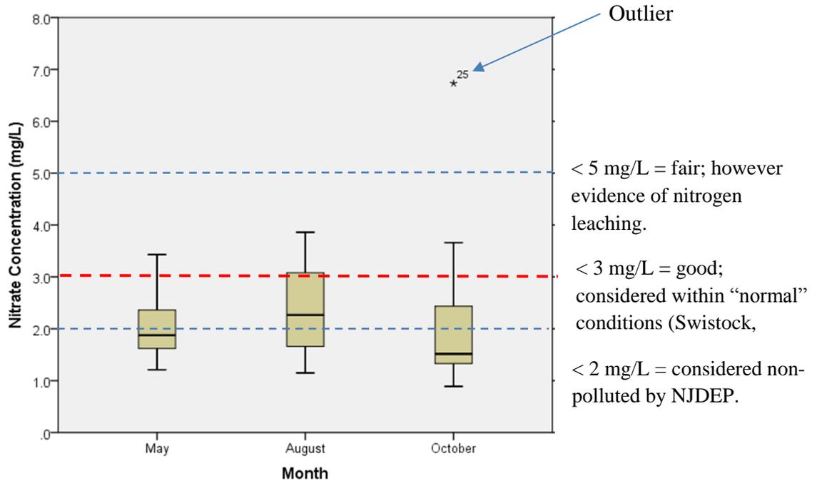
**Figure 3:** Box plots of average nitrate ( $\text{NO}_3^-$ ) concentrations for all locations at one foot water depth. Data collected from 2004 – 2016.
